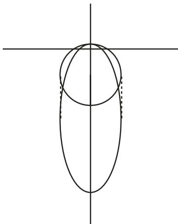
In designing an oval guard for a Bowie, the same process is used. The height and width of the guard is designated, then a center line and two horizontal lines for the spine and bottom of the riccasso are placed on the pattern.
