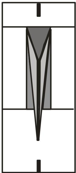
The line from the bottom of the riccasso is transferred around to the back of the guard material. And then another line is marked  $1/32"$  (.031) below it to indicate where the guard will be milled to for the finger relief area.
