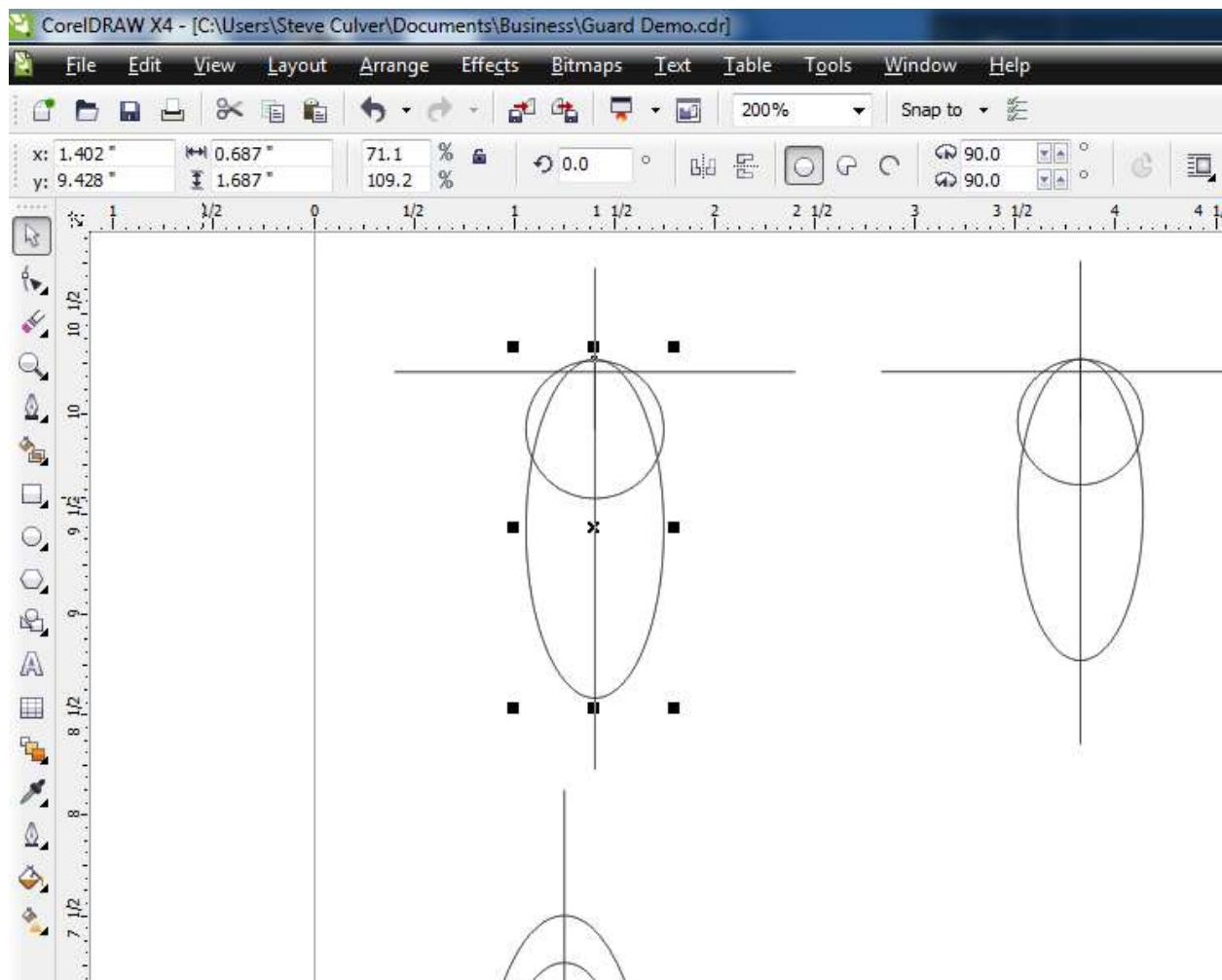
My hunter guards are designed using an oval to designate the bottom of the guard and a circle of the same diameter that the oval is wide for the top of the guard. When sawing and grinding the guard out, the material is removed in a straight line along the edge of the circle and oval.
