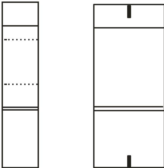
Using a 1/2" (.500) end mill, the guard material is cut away to the line that is 1/32" below the riccasso bottom mark.
