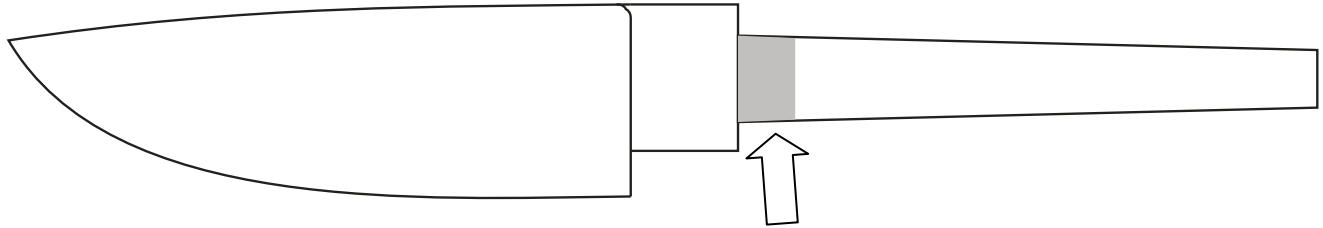
When grinding the tang, do not grind the 1/8" of the tang behind the riccasso. This area is finished at the same thickness as the riccasso and will be filed to press fit in the slot in the guard. I file this area to be .002" thicker than the guard slot is wide.
