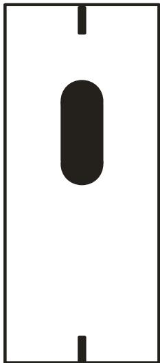
As I fit the guard to the tang, I square out the ends of the slot by using a file that has had one side ground "safe". The "safe" side of the file is held against the side of the slot as it is used to remove the radius' at the ends of the slot.
